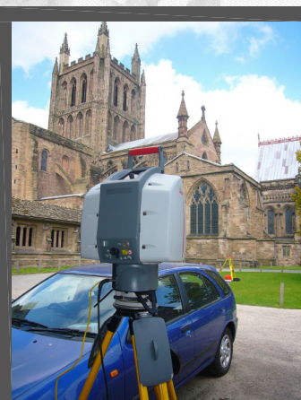
Leica HDS - Hereford Cathedral Laser scanning in 2008
