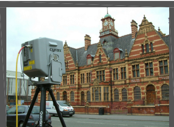
Leica Cyrax 2500 - Victoria Baths Laser scanning in 2003 BBC2 TV
